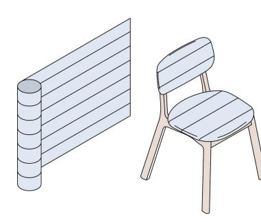
This means fabric is cut across the roll and selvage is on top and bottom.
